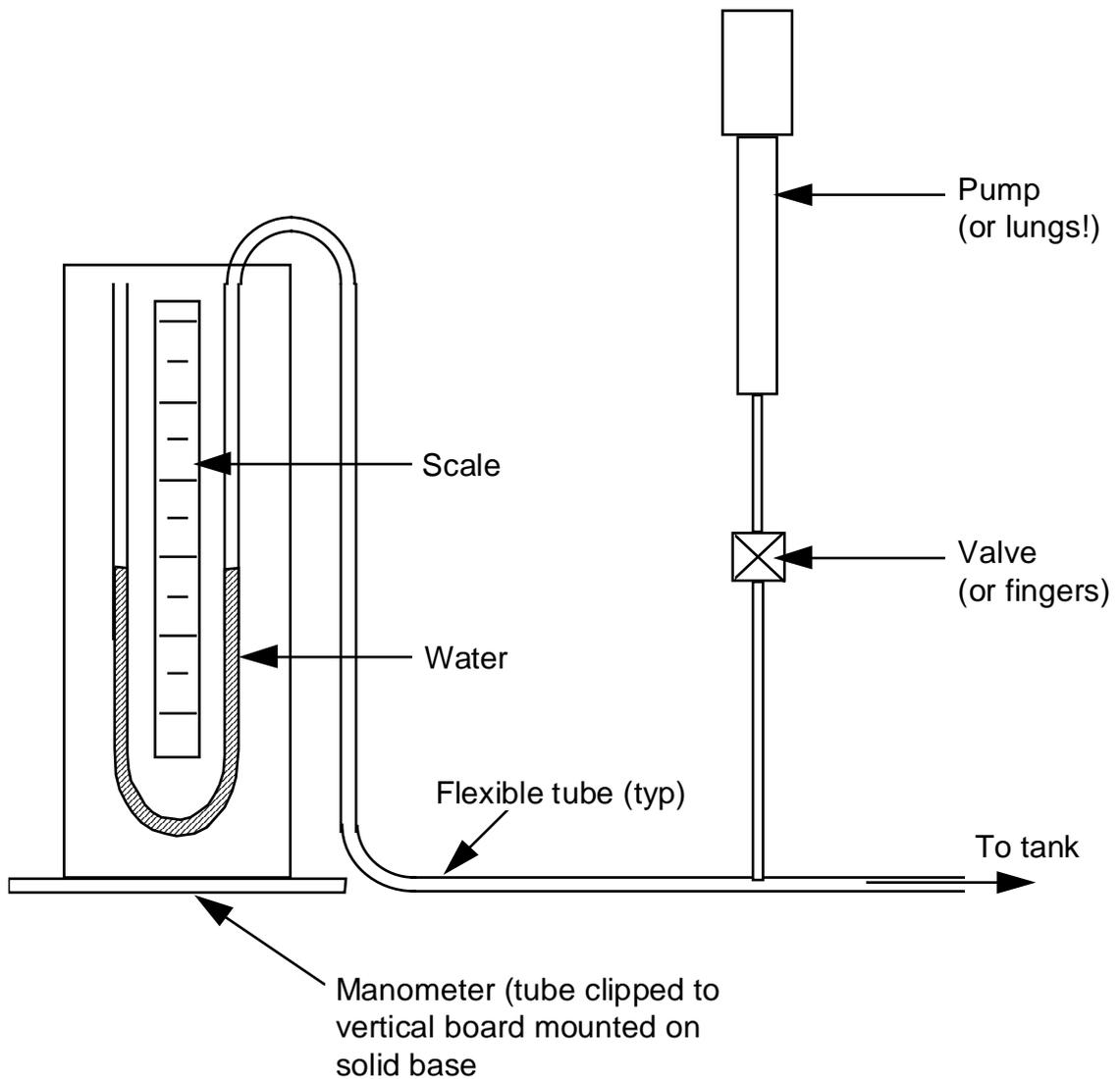
Measuring Equipment: Manometer, flexible tube, drilled bung/hatch cover, pump, valve, stop watch.
