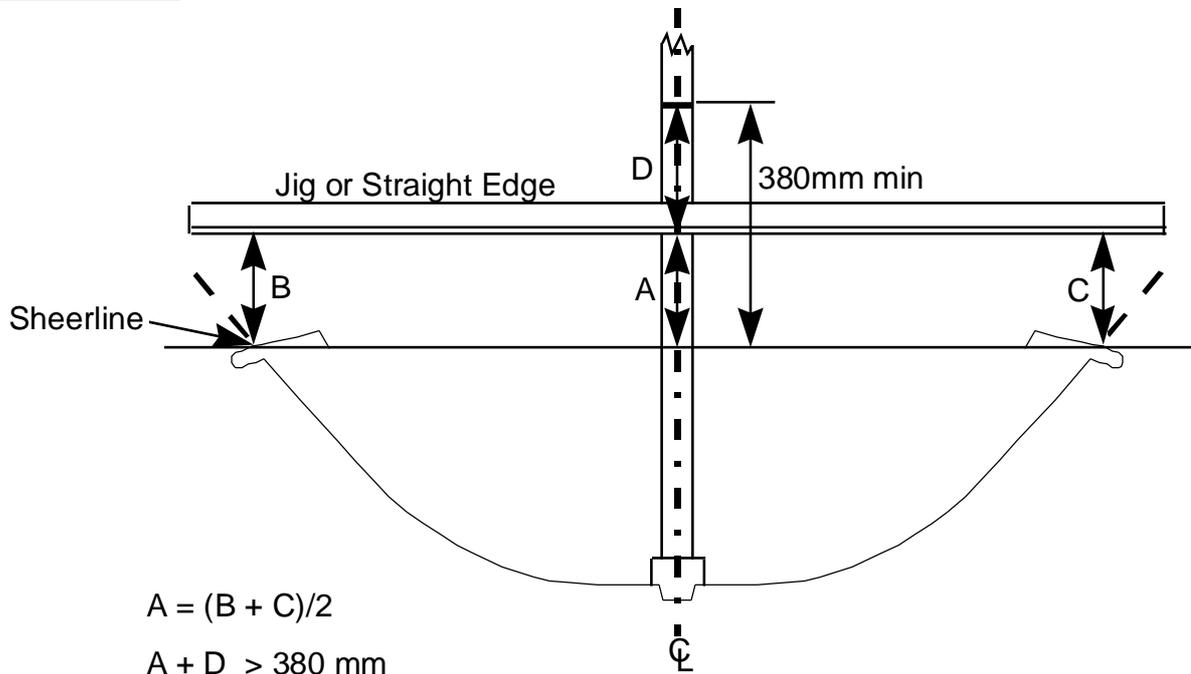
Measuring Equipment: Sheerline jig, masking tape, pencil, 2.5m straight edge or straight edge jig with moveable legs, 150 or 300mm rule, tape measure, scribe, thin indelible felt pen.
