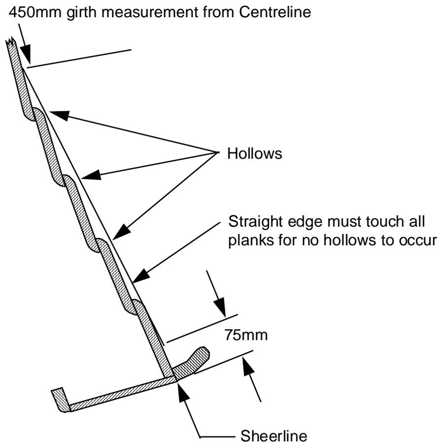
Measuring Equipment: 0.75m straight edge, 150mm rule, tape measure, Sheerline jig/masking tape/pencil, (thin string).
