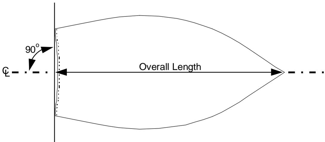
Measuring Equipment: Long tape measure, Long spirit level, Water tube, levelling equipment (e.g. Car jack & launching trolley), Straight edge longer than Transom width, 2ft straight edge, Waterproof tape or crayon, buoyancy test weights.
