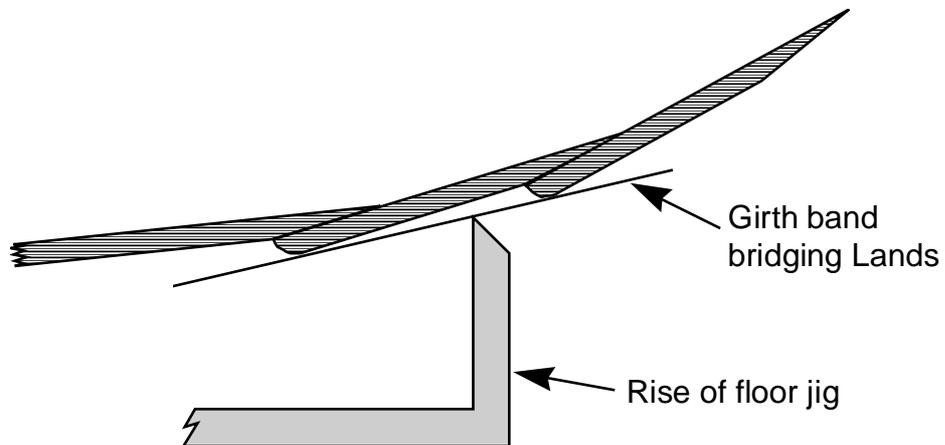
Measuring Equipment: Rise of floor jig, masking tape, pencil, tape measure, spirit level.
