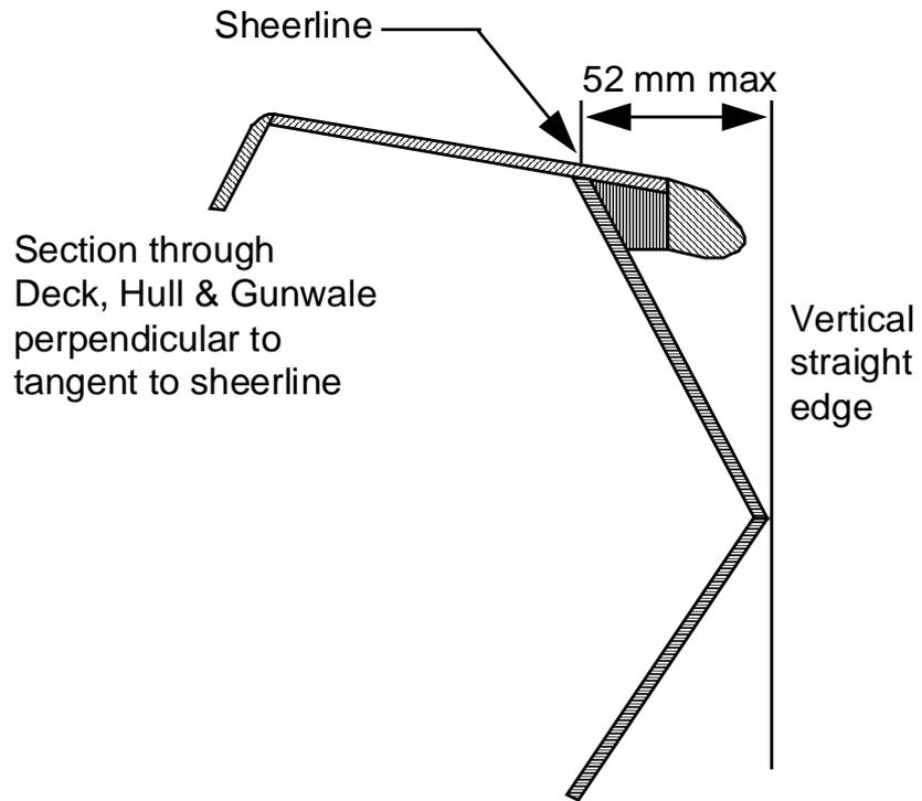
Measuring Equipment: Sheerline jig, masking tape, pencil, Gunwale Width jig or adjustable square with levelling bubble, small spirit level, 0.75m straight edge, 150mm rule.
