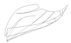
To this spine a 'single plank per side' is attached and the thoroughbred shape created simply by seaming the two contra-curving overlapping darts.
