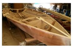
Fyne Boat Kits of Cumbria have developed an innovative patented construction approach to a design by Cumming utilisina Colin ockoume marine boowylg and solvent free epoxy to create a strong durable lightweight ecologically sound aesthetic craft.
